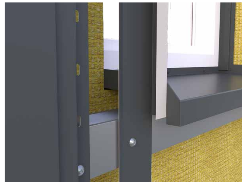
Illustration 96 • Montering holdevinkel lysningspanel
